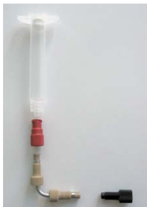
figure 14 Mounting view of the barrier seal module
